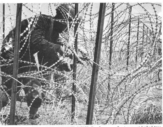
CONQUERING CONCERTINA WITH DETERMINED SHEARS. Two "aggressors" cut away at barbed tape entanglements with bolt cutters to establish how long it would take to breach such a barrier. Barrier Technology Handbook, just published by Org. 1711, contains data on this and wide variety of other barriers. See page 8 for story and photos.
